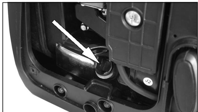
5. If the oil is below the Min. level on the dipstick, top up the oil reservoir with fresh oil.
