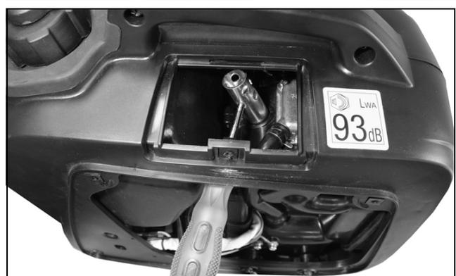
6. Check the spark plug gap (a) with a feeler gauge, it should be between 0.6 and 0.7 mm.
