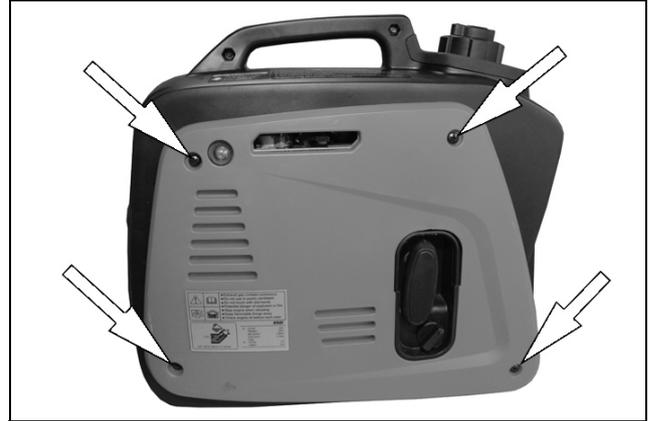
2. Remove the air filter cover screw.
