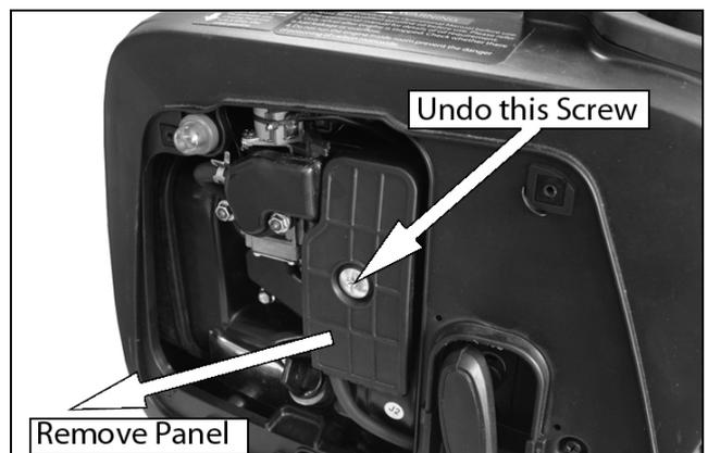
4. Remove the air filter element.
