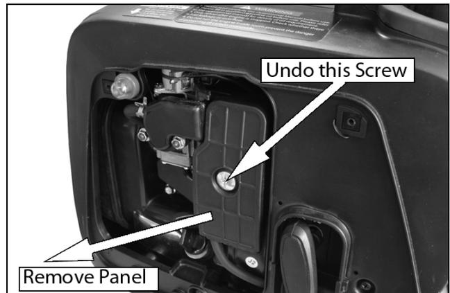
4. Remove the air filter element.
